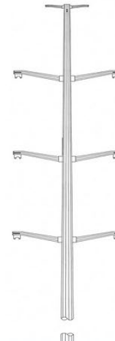
138 KV Self-Supporting Tublar Steel
